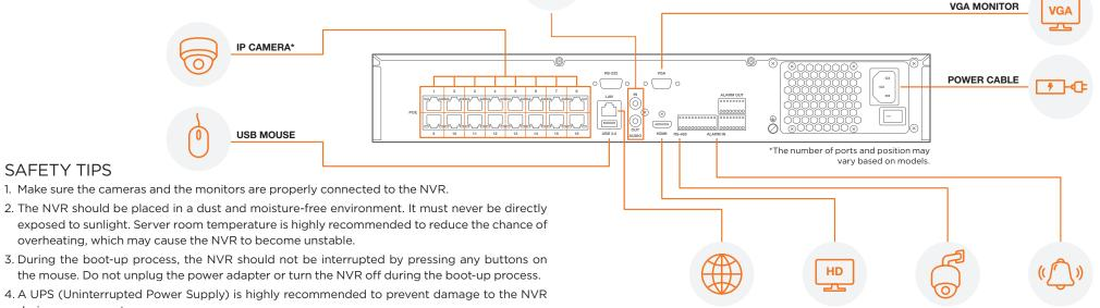
recommended ambient temperature of 104°F (40°C). To prevent airflow restriction, allow at least 3 inches (7.6 cm) of clearance around the ventilation openings.
