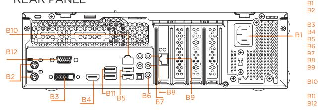
AC power socket PS/2 keyboard and PS/2 mouse ports DVI-D port True HD port 2x USB 2.0 ports Mic in (pink) Line out (green) Line in (blue) Ethernet port to the camera network Ethernet port to the local network USB 3.0 ports
