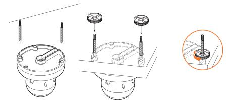
the camera module. Tighten the screw once the adjustment is complete. Remove the protective film from the lens cover. Softly wipe the dome with lens tissue or a 6. microfiber cloth to remove any dust or smudges left from the installation process.
