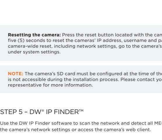
**Resetting the camera:** Press the reset button located with the camera's cables for five (5) seconds to reset the camera's IP address, username and password. For a camera-wide reset, including network settings, go to the camera's web interface under system settings.
