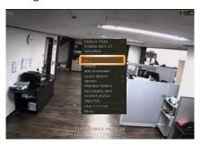
PTZ Control: In PTZ mode, the user can control the PTZ camera using the USB mouse. While pressing the left button, drag the mouse cursor up/down or left/rightward to move the camera's pan/tilt position. The further away from the center the mouse's cursor moves, the faster the PTZ camera will move. To move the camera to a preset position, click the preset position number at the bottom of the screen to move the camera accordingly. The presets must be set before selection.
