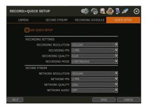
Users can setup recording resolution, FPS, quality and mode on recording settings.
