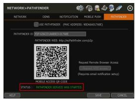
Check the PathFinder status at the bottom of the screen to complete the setup. STATUS will display "PATHFINDER SERVICE IS STOPPED" or "PATHFINDER SERVICE ACTIVATED" according to the system's status.
