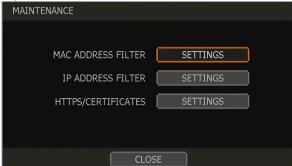
MAC ADDRESS FILTER: Blocks or allow specific Mac addresses from a C3 client or mobile app from accessing the DVR.
